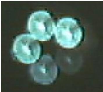
The "stars" are about 180" ( about 3 arc min) in diameter. The picture matches the spherical aberration expected from an f/2 mirror fairly well.
