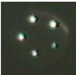
The smallest (0.9") "star" is about 25" (about 0.42 arc min) in diameter. It is likely that better collimation of the test setup would have reduced the spot size further. Also, a custom corrector would be beneficial.
