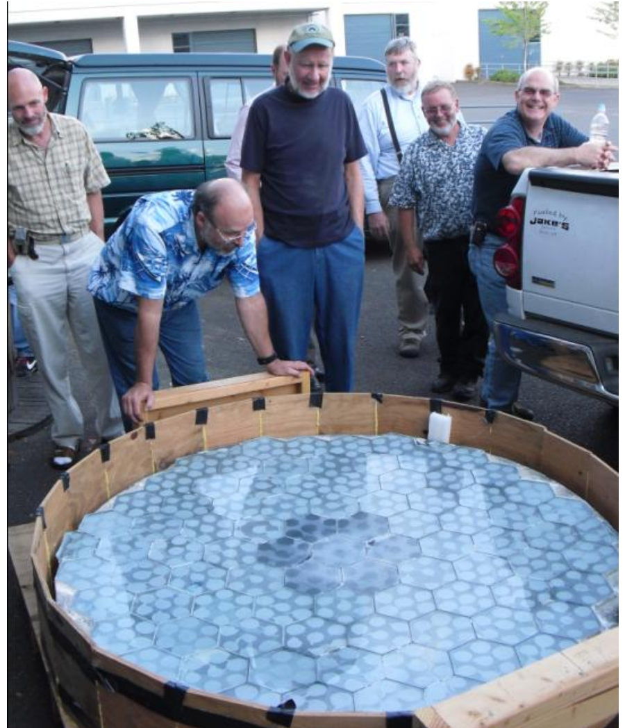
David Davis's 60-in. tessellated glass over foamed glass (D.D. with suspenders, Russ Genet with hat)
