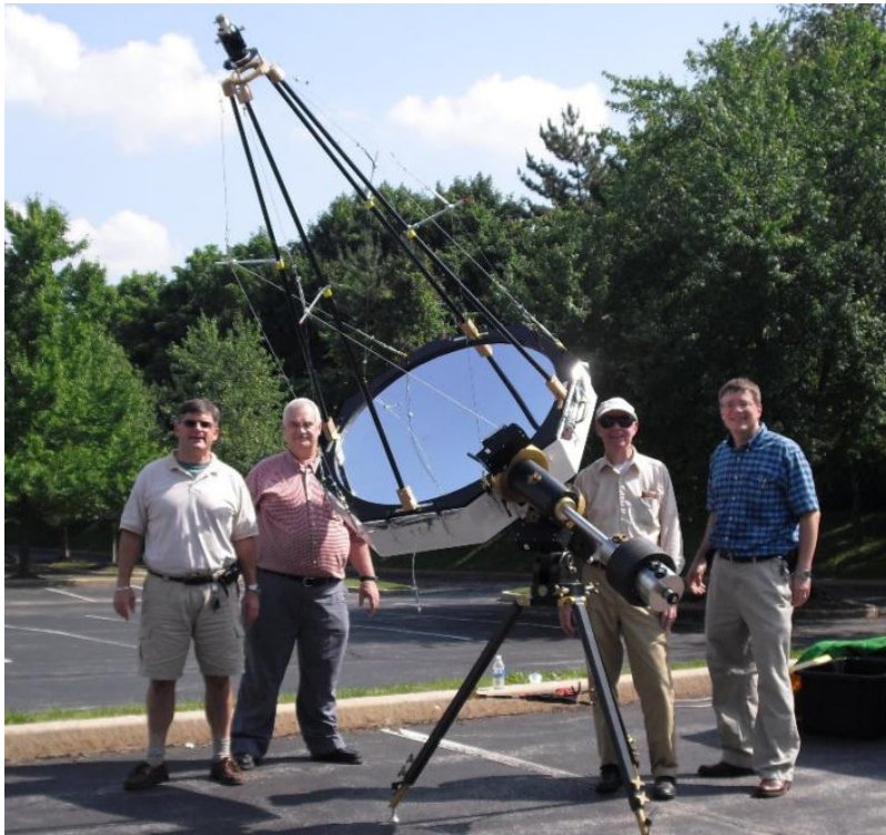
42-in. scope with Gravic high-speed photometer
