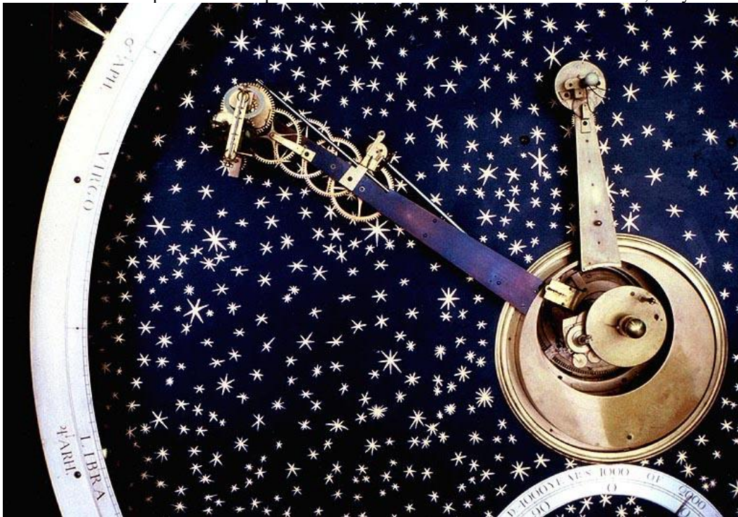
Fig. 17. A view of a portion of one Rittenhouse orrery – it's really a partial mechanical almanac. The steel ring engraved with the months and constellations and the longitudes of assorted orbital nodes is about 2 inches in width while the display inside this ring has a diameter of about 42 inches. Rittenhouse himself did not make the mahogany case which actually cost him 60% of his fee. The model for Saturn is directed to about 10 o'clock while that for Jupiter is aimed to almost 12 o'clock. Earth and Moon are just barely visible at the edge of the small brass disk to the right. The background star pattern is idealized.
