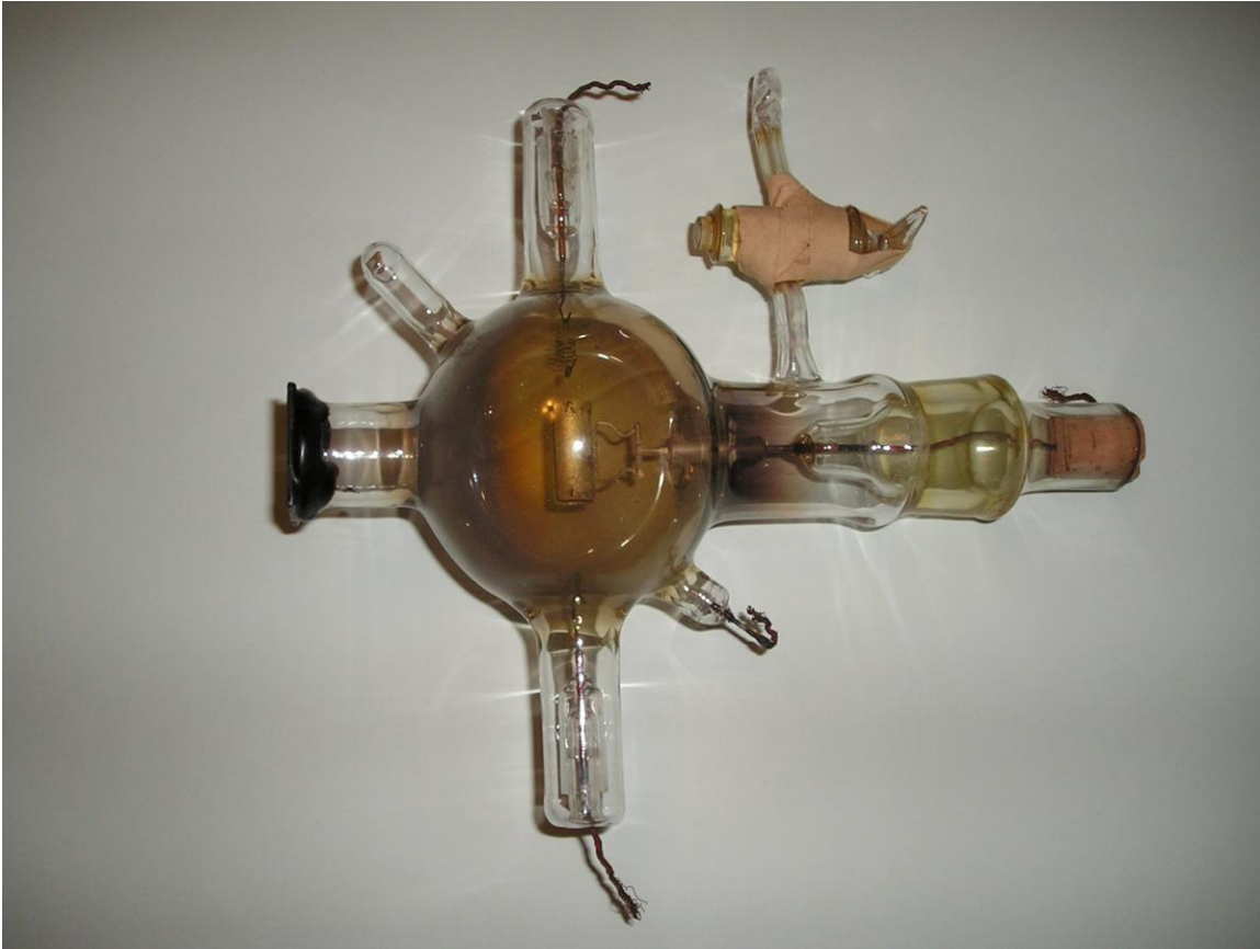
Fig. 34. This Geiger-Müller tube is somewhat more complex than the one used by Mohler to measure far-UV solar flux but is basically similar to his device. The square quartz window to the left is about 1.25-inch on a side; the black deposits are just sealant. The photocathode is presumably gold and possibly the coloration of the inside of the glass is also sputtered gold. All the electrical connections are intact and the electrical leads show clear signs of attachment to other circuit elements. The stopcock is held closed by a 1930s bandage.
