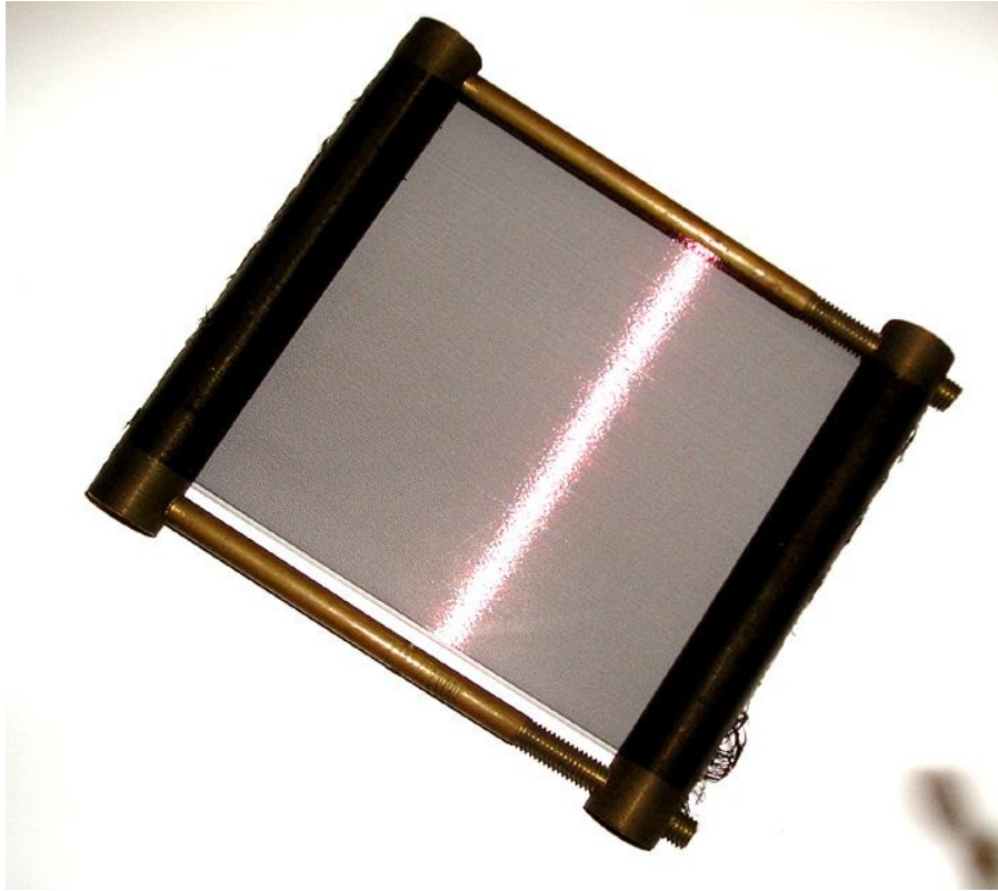
Fig. 5. The brass frame is about (5.5 x 5)-in and the thicker rods were worked on a lathe so as to cut a 0.02-in thread along their lengths. Across the frame and held taut in the threads there is wrapped a continuous 0.01-in diameter wire. Light from celestial sources passes through this coarse, old-fashioned grating onto the objective of a telescope and is then imaged into the telescope's focal plane where it appears as a spectrum from each source. The bright streak across the wires is glare from the ceiling light above the camera that was used for this picture. Modern versions of this device have microscopic grooves (the analogues of the wires) ruled into transparent or reflecting surfaces.
