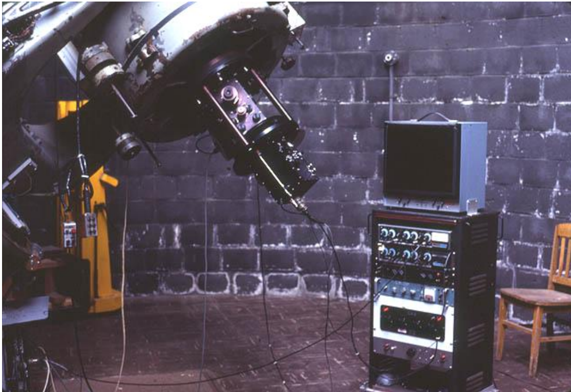
Fig. 48. The device known as the PEMP mounted on the reflector. This was its appearance after moving to a Kemp-type photoelastic modulator that would yield simultaneously the Q , U and V components of the net polarization vector. All electronics are in the floor rack and the monitor would show the data string in real time. The archiving computer is in the adjoining warmed room. The yellow object in the background is a forklift used to remove and re-install the paraboloid and its cell. Obviously, the walls need pointing and painting at this time.
