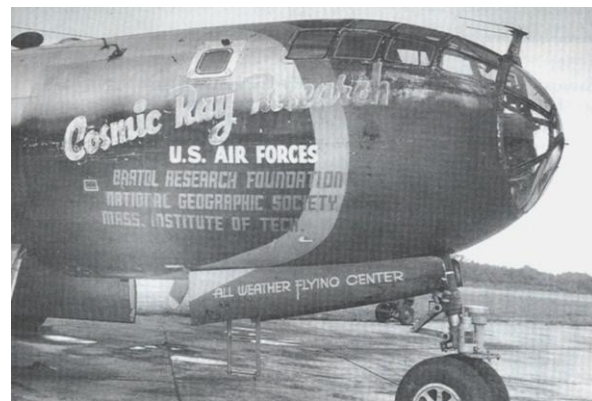
Fig. 2. A disarmed B-29 modified for cosmic ray observation at about 40,000 feet.
