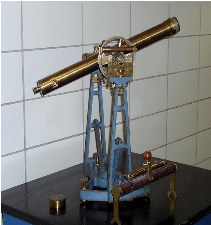
Fig. 4. A portable transit made in 1886. One of the cylindrical pivots can be seen riding in its bed with a small spirit level above it and another larger level is upright on the table.
