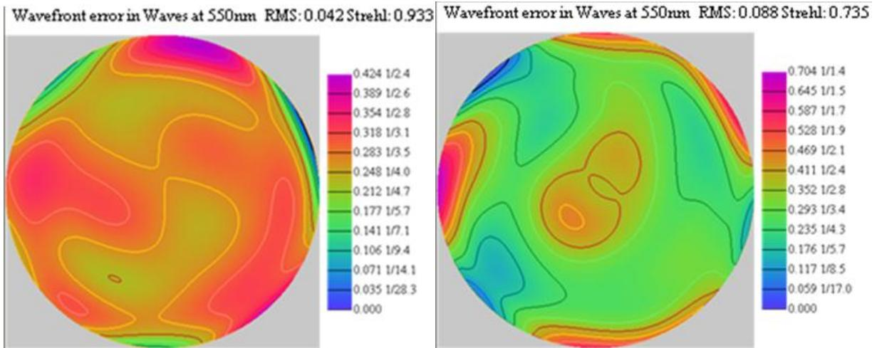
The above example compares mirror 5 before coating (left) and after silvering and overcoating with extra-thin Permalac (right). The silvering steps removed the edge orientation mark and so the image on the right has to be rotated CW about  $90^\circ$  to match the orientation of the image on the left. The RMS surface height aberration increased from 0.042-waves (@550-nm) to 0.088-waves.
