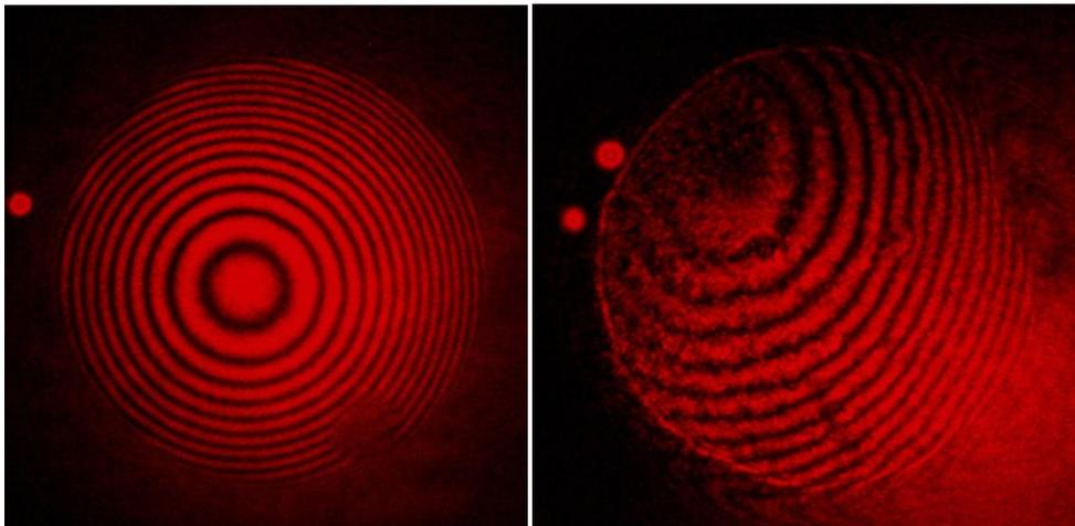
On the left is an interferogram of mirror 20 which was silvered but not overcoated. On the right is mirror 5 which has the extra-light Permalac coating. High-frequency, low amplitude, aberration is evident by the lack of smoothness of the fringes.
