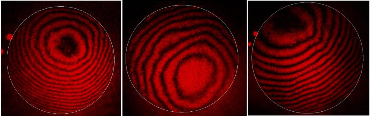
Interferograms of mirrors 9, 23, and 25 (from left to right) are shown above. There is some evidence of surface ripple or running in the ETT overcoat. Overall, the surface smoothness is better than for the Phase II mirrors.
