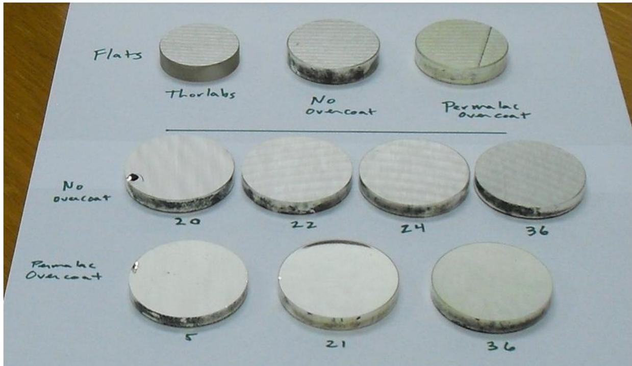
The middle row consists of four silvered concave mirrors. The bottom row has the extra-thin Permalac coated mirrors. A slight yellow tinge is also evident in this set.
