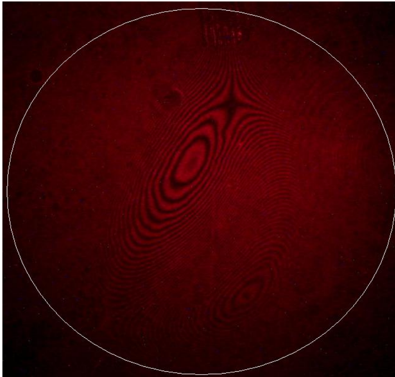
Rotated, 90 degrees CCW from the front, and the astigmatism rotated too. Notice the high spot in the lower right corner.
