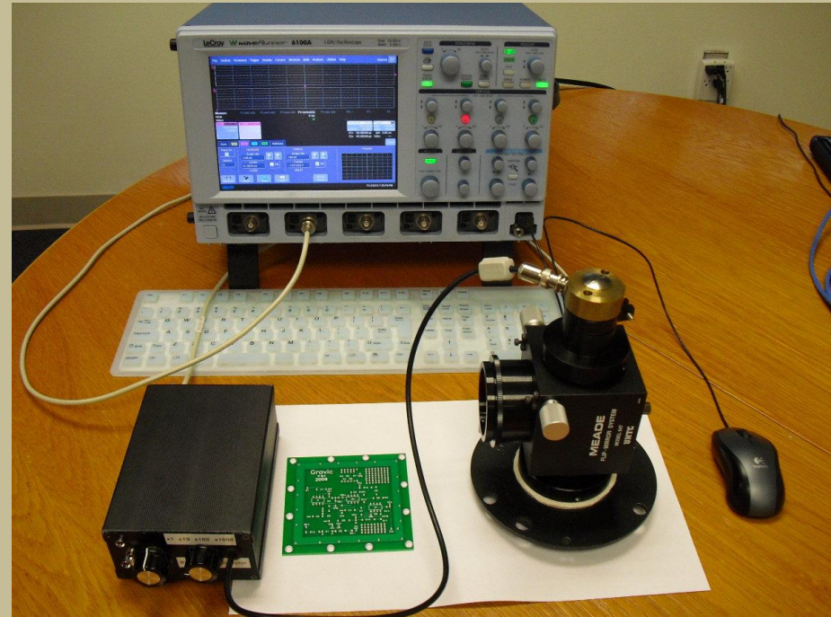
High-speed Si detector/trans impedance amp at Gravic
