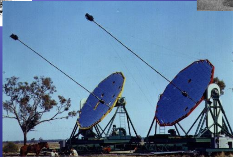
Hanbury-Brown Intensity Interferometer 6.5-m
