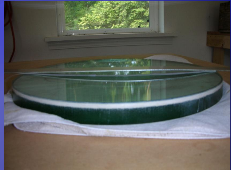
Mel Bartle's 13" soda lime slumped meniscus mirror
