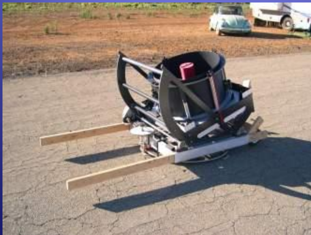
Everything but the truss tubes stacked as a wheel barrow - Howard Banich 28 inch alt-az
