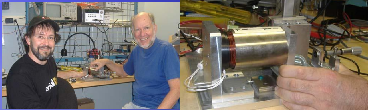
One of the 120 Gemini voice coil actuators
