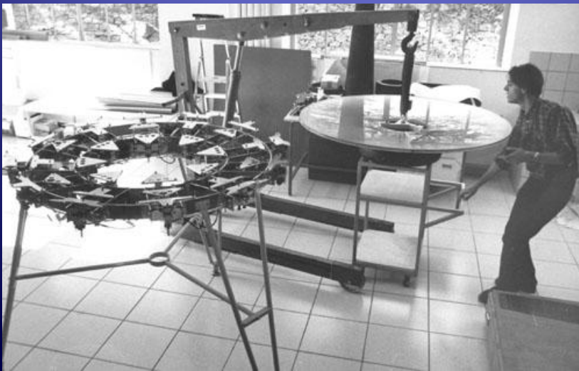
French ATM with 1-m meniscus mirror and astatic support system
