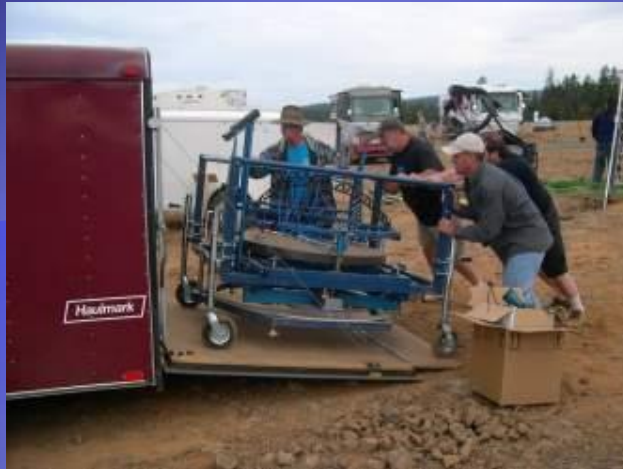
Everything but the truss tubes stacked and rolled on wheels – Dan Bakken's 41.2 inch String Alt-Az
