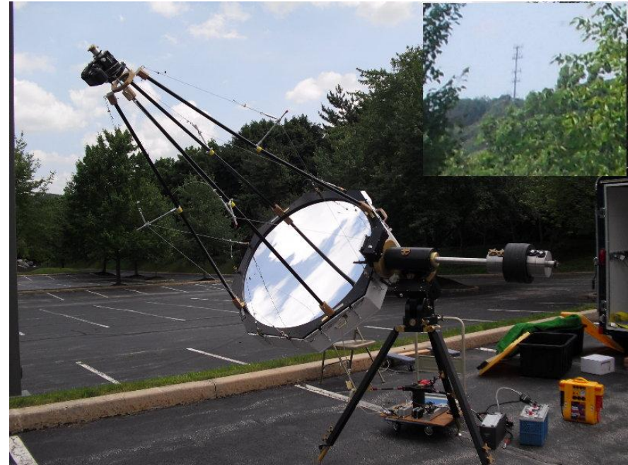
42-inch pneumatic mirror prototype at Gravic Labs
