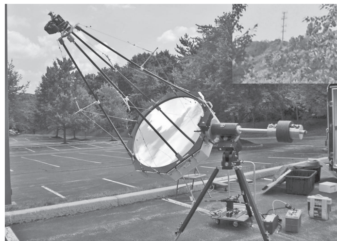
Figure 4: A 42 inch cell and OTA mounted on an IPI393 GEM mount. A daytime image showing a near field of trees and a distant one of a structural tower is shown in the upper-right insert. The camera in automatic mode had difficulty deciding which fraction of the scene to focus on. The piecrust distortions around the edge of the image result from failing to re-tension the film in its cell. Stratified inversion layers above manmade structures account for the ragged tower image. In order to facilitate development testing, the inside cables on the truss members are not in place here and this condition caused the truss poles to bend inwards.
