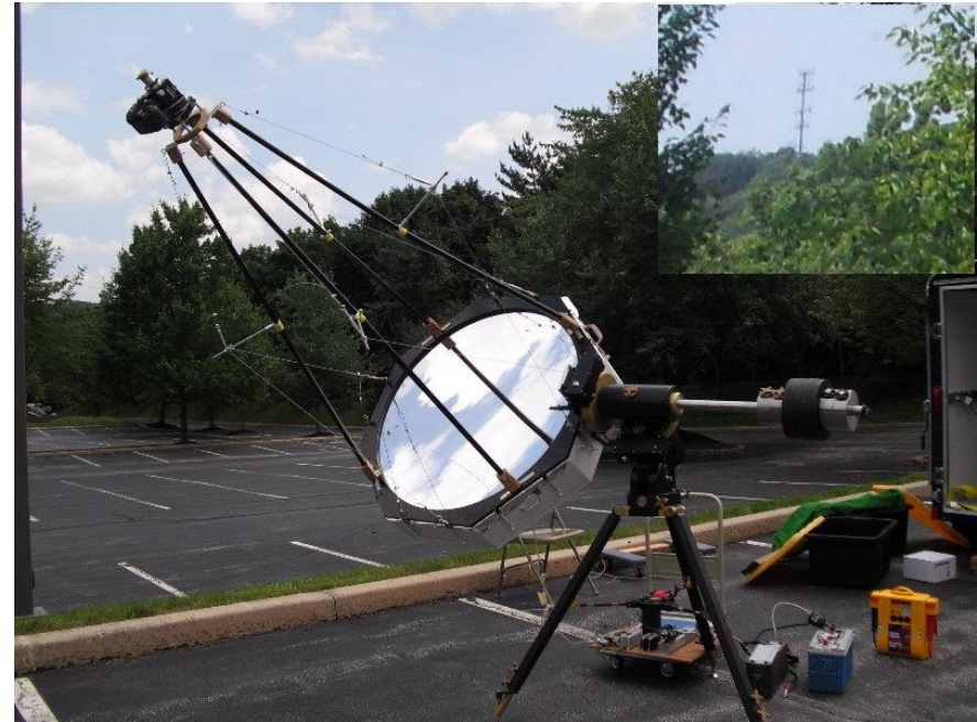
42-inch pneumatic mirror prototype at Gravic Labs
