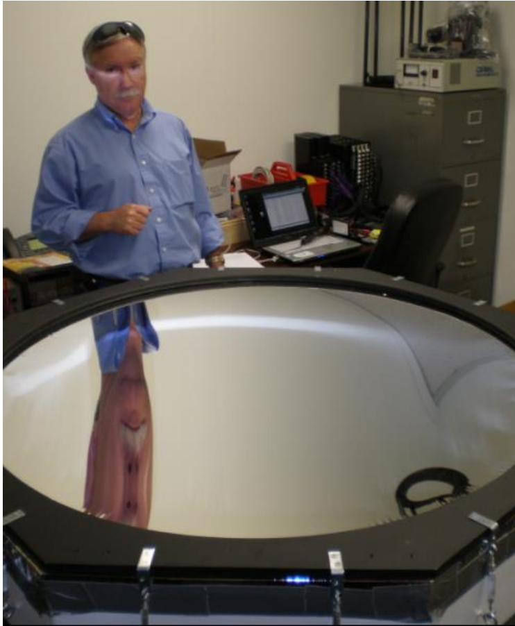
Properly tensioned membrane
