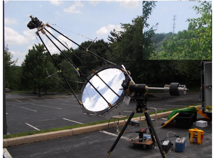
Flux collector - Pneumatic Mylar Mirror Telescope at Gravic
