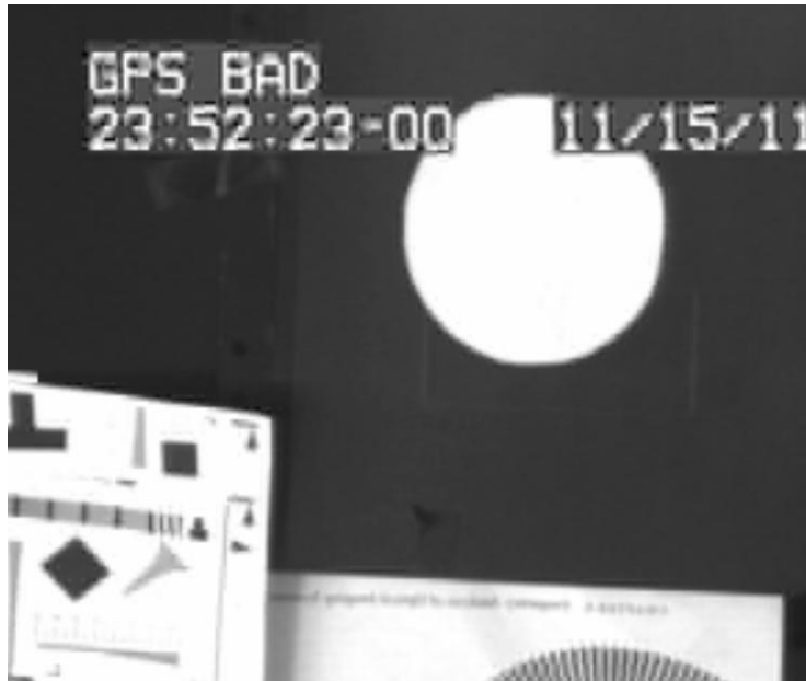
Figure 8. Image of the test target with no flat in use (aimed directly at the target).
