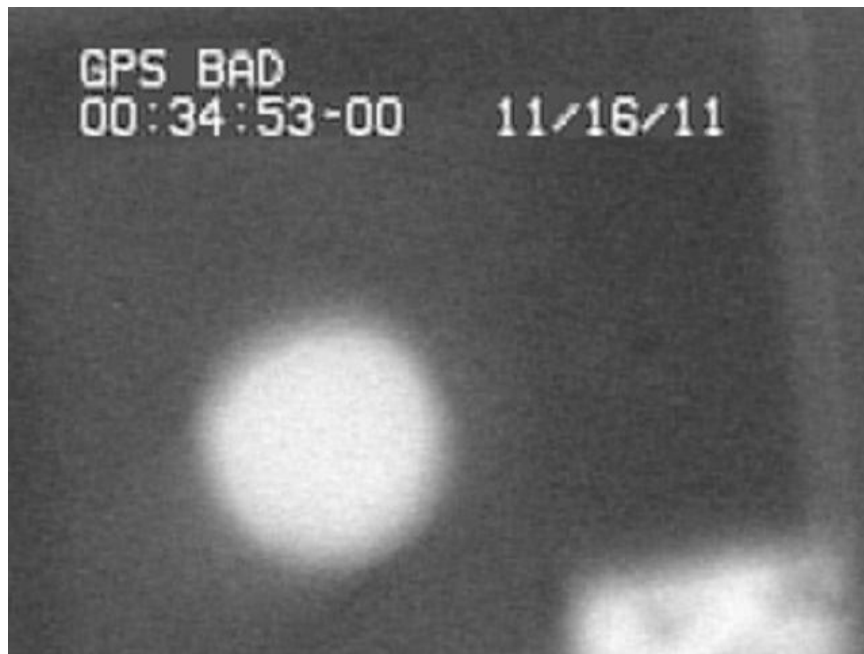
Figure 11. Image from light reflected off a 60 mm diameter region of the BLB-31.3 flat. Overall reflectivity of this flat was much higher. Aberrations limit the resolution of the image to about one arc minute.
