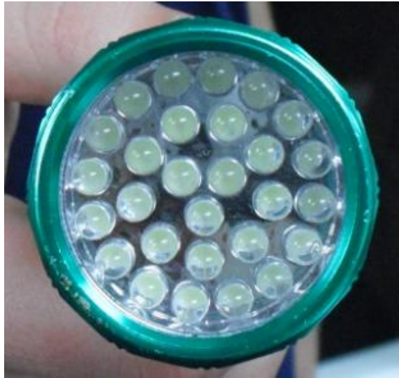
Figure 15. 1.75" diameter LED flashlight source for spin-cast mirror test.
