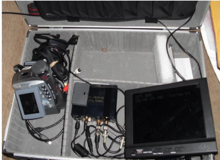
Figure 7. Video recording equipment. The Canon DVR, GPS time insertion device, and monitor are seen.
