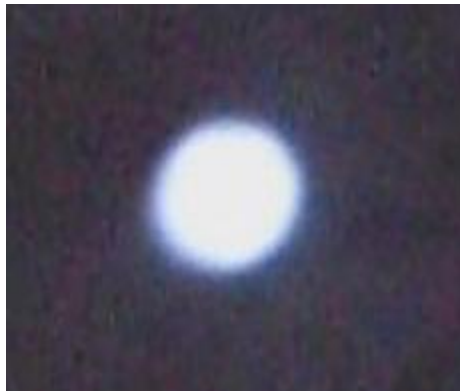
Figure 16. Returned image from the spin-cast mirror. Some astigmatism is apparent. Mainly, the individual LEDs are not visible presumably due to the high-frequency ripple. The resolution is about 3 to 5 arc minutes.
