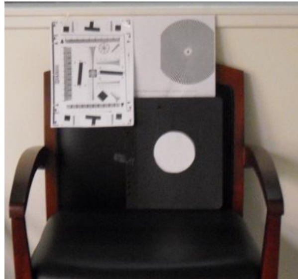
Figure 6. The white test spot is 4.5 inches in diameter so it subtends 1031 arc seconds at the flat under test (17.2 arc minutes).
