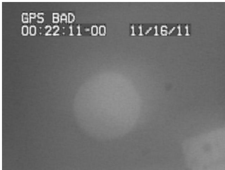
Figure 10. Image from light reflected off a 60 mm diameter region of the BLB-31.2 flat. Aberrations limit the resolution of the image to about 20 to 30 arc seconds.
