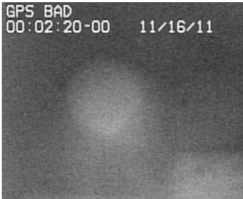
Figure 9. Image from light reflected off a 60 mm diameter region of the BLB-31.1 flat. Aberrations limit the resolution of the image to a couple of arc minutes.
