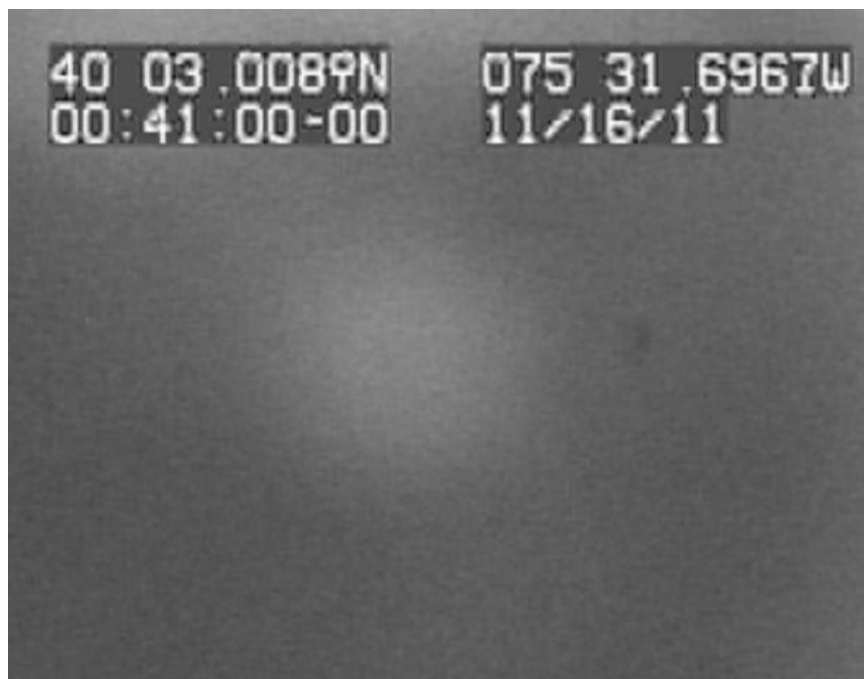
Figure 12. Image from light reflected off a 60 mm diameter region of the BLB-31.4 flat. Aberrations limit the resolution of the image to about 5 arc minutes or worse.
