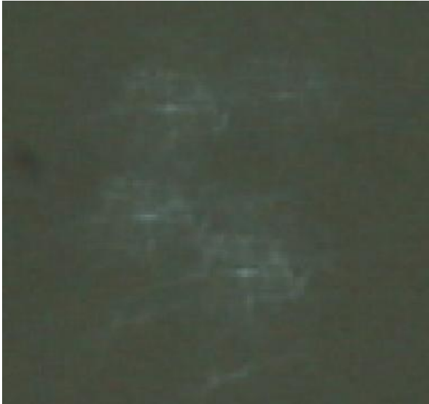
Subjective best focus of the Hubble test source at 11-m.
